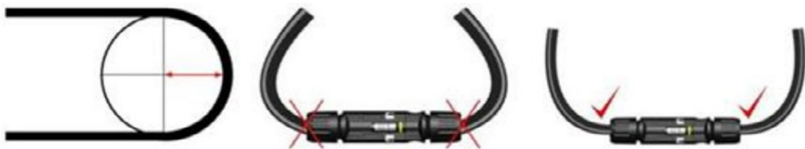
FIGURE 7-2 MINIMUM BENDING RADIUS OF THE CABLE
