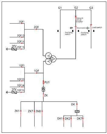
Figure 5-1 The switch status before maintenance
