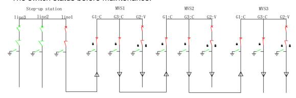
Figure 5-3 The switch status before maintenance:
