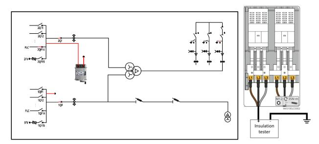
Figure 4-16 Test diagram of low-voltage cabinet D2
