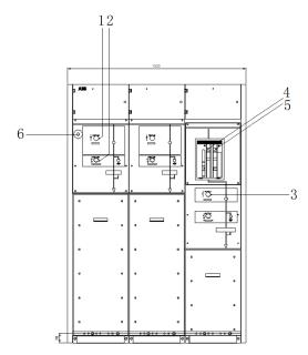
Figure 2-14 Ring main unit SAFE 40.5 CCV appearance
