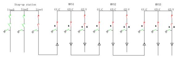
Figure 5-5 the switch status before maintenance
