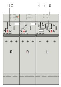
Figure 2-15 Ring main unit 24kV RRL appearance
