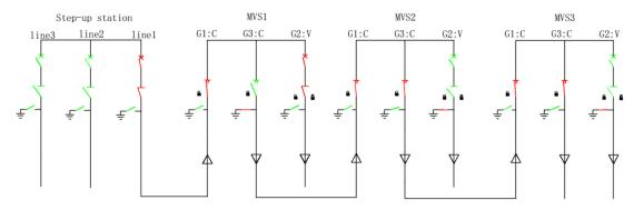
Figure 5-4 the switch status after maintenance
