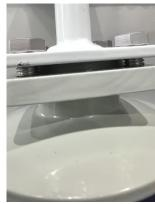
5) Remove the oil cup and fill the cup with oil level between the two red lines.
