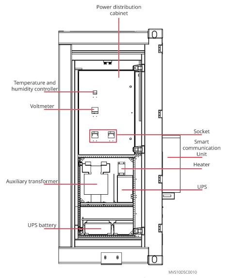
Figure 2-17 Power distribution cabinet front view layout Figure
