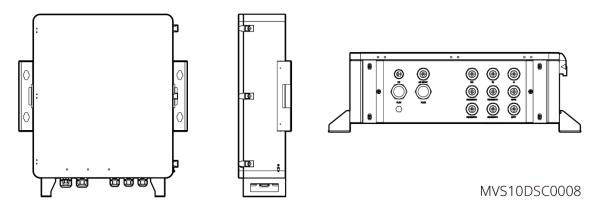
Figure 2-18 Smart Communication Unit appearance
