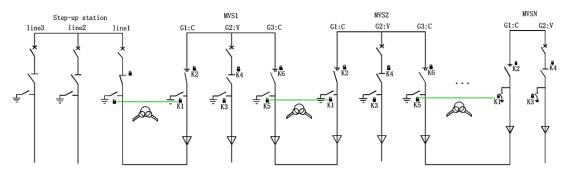
Figure 4-5 CVC type ring main unit normal interlocking
