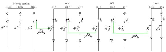
Figure 4-10 The A3 interlocking of the CCV ring main unit
