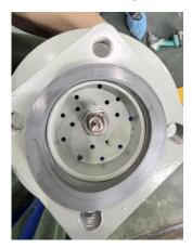
4) Install the respirator to the breathing tube port, tighten the bolts diagonally, and install the sealing gasket as shown in the following figure.
