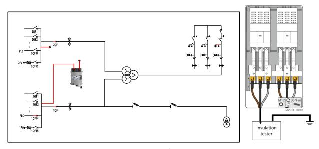
Figure 4-15 Test diagram of low-voltage cabinet D1
