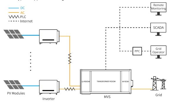
Figure 2-1 MVS Typical Application Diagram
