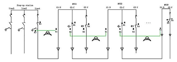
Figure 4-8 The normal interlocking of the DCV ring main unit
