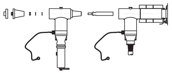
Figure 5-9 Lightning arrester and separable insulating sleeve
