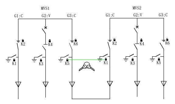
Figure 4-3 The normal interlocking of G1 cabinet with load switch
