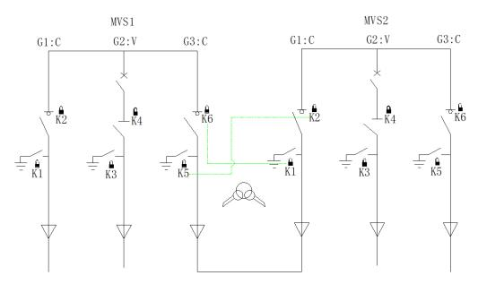
Figure 4-12 P1 Interlocking
