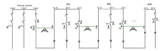
Figure 4-7 The normal interlocking of the DVC ring main unit
