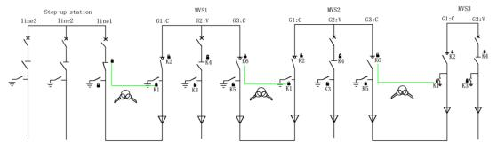
Figure 4-11 The A3 interlocking of the CVC ring main unit
