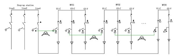
Figure 4-4 CCV type ring main unit normal interlocking
