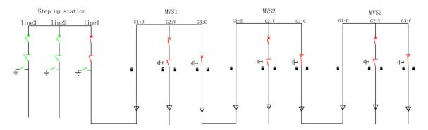
Figure 5-7 The switch status before maintenance
